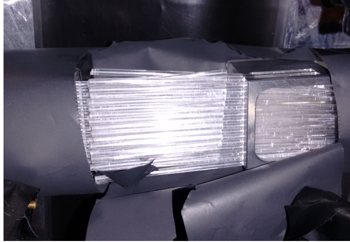
Figure 5.17: Loose fibers in the central region where the electrons hit ARGUS. Picture was taken after the test beamtime.
