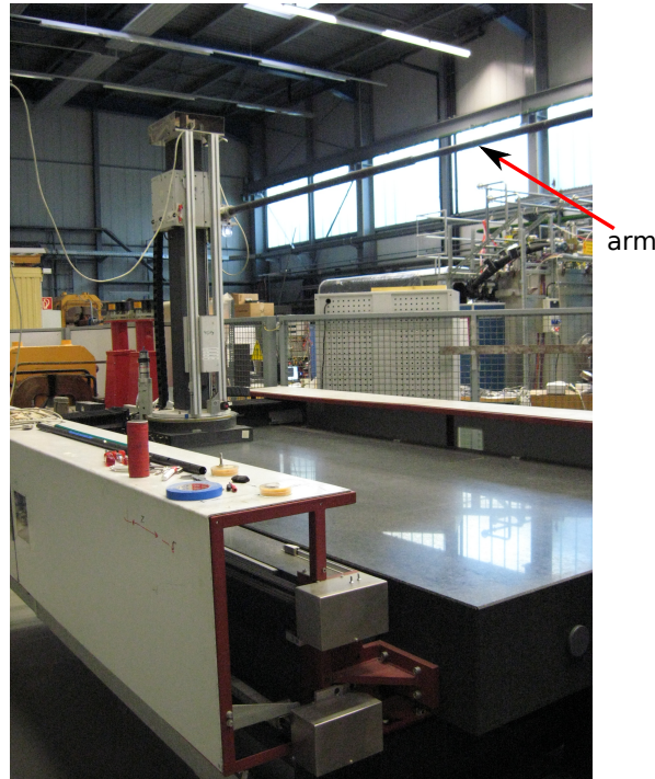
Figure 3.2: Field measurement setup at the GSI. The 3 Hall probes are located at the end of the 3 meter long arm [Han].
