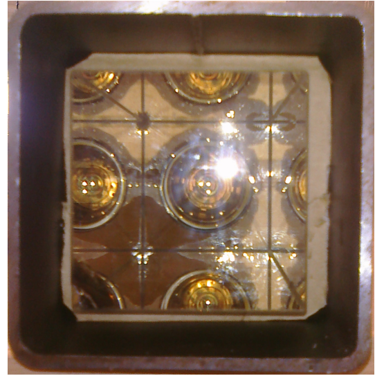
Figure 5.8: GIM prototype front view, without cover. The lead glass is placed in the iron tube with a paperboard stand and through the lead glass, the photo cathode of the photomultiplier is visible.
