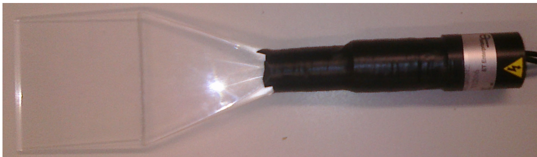
Figure 5.16: The light guide is attached to the photomultiplier with black tape.
