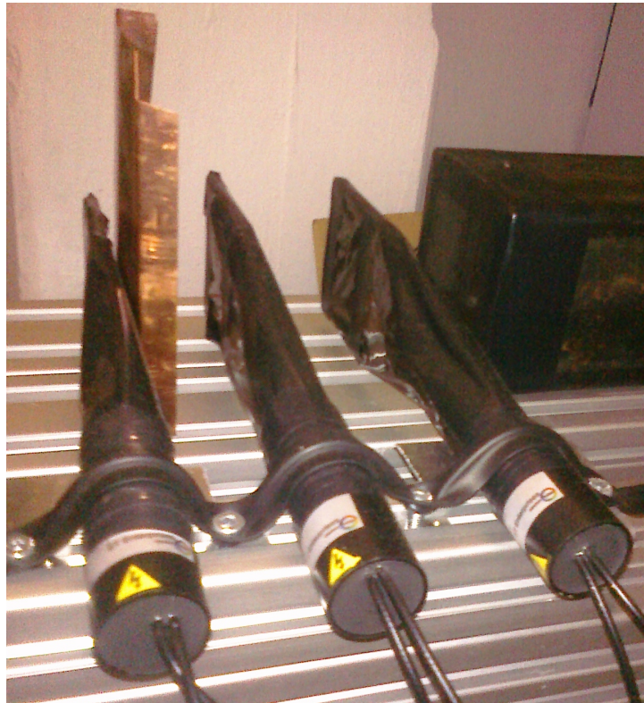
Figure 5.17: The prototype of the FluMo detector installed in the experiment, the copper plate was used to test the difference with and without converter.
