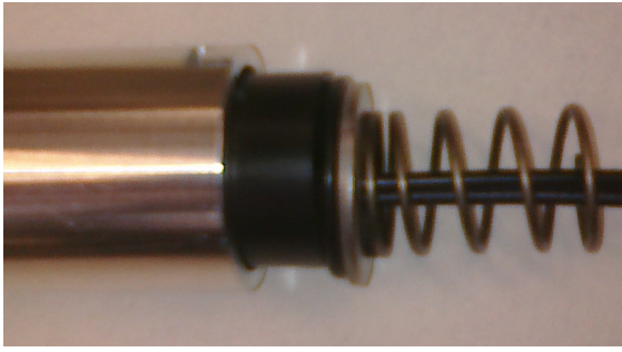
Figure 5.19: All FluMo parts put together in the right order. The O-ring seal guarantees light tightness, the steel washer protects the base from the pressure of the spring.
