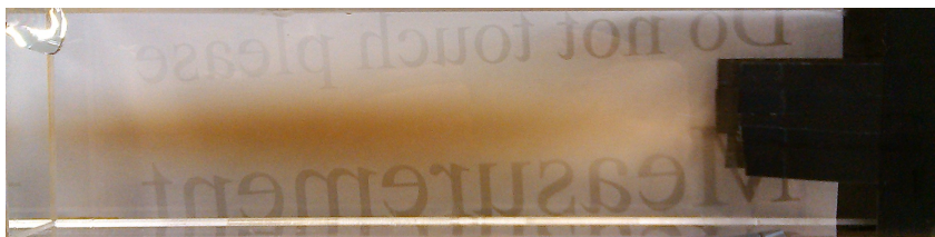
Figure 6.12: Lead glass of the GIM prototype after the irradiation.
