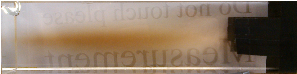
Figure 5.2: Lead glass with brown color from radiation damage.
