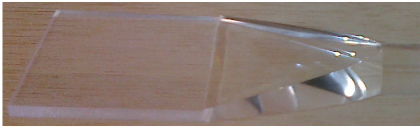
Figure 5.15: The scintillator is glued to the light guide with superglue.
