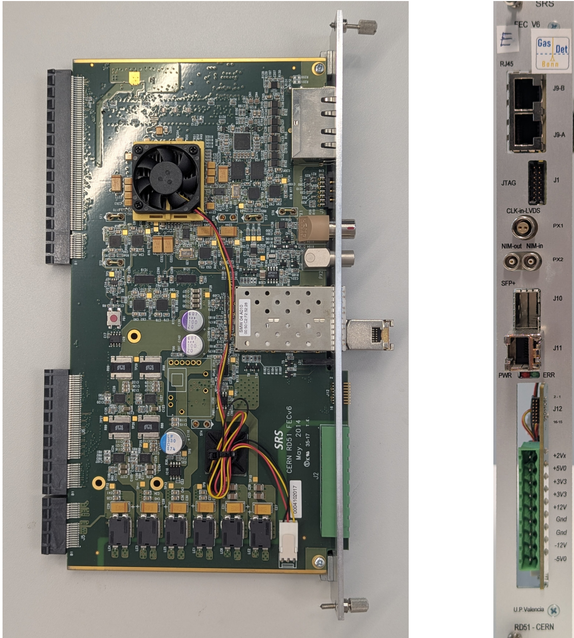
Figure 2.2.: Side (left) and front (right) view of the FEC. All ports on the front panel are labeled. J1 is the JTAG port. PX2 are the NIM input and output. J11 contains a pluggable network interface for the Ethernet connection to a computer. J12 is an additional connector accessible from the FPGA. The large green 9-pin port is used to connect the power supply. The FPGA sits under the black fan visible in the side view.
