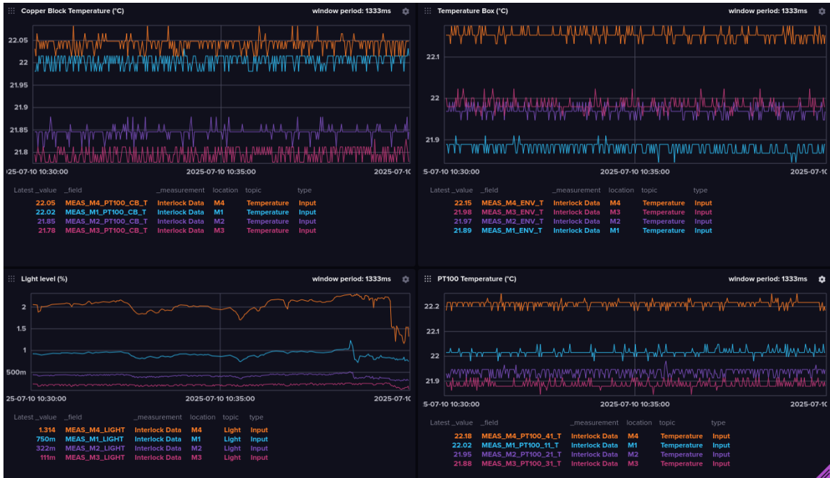
Figure 4.17: Different sensor readouts displayed in the Influxdb like the copper block temperature, aluminum block temperature, general box temperature and the light level. The measurements were conducted with no device or cooling in the box and with the lids closed.
