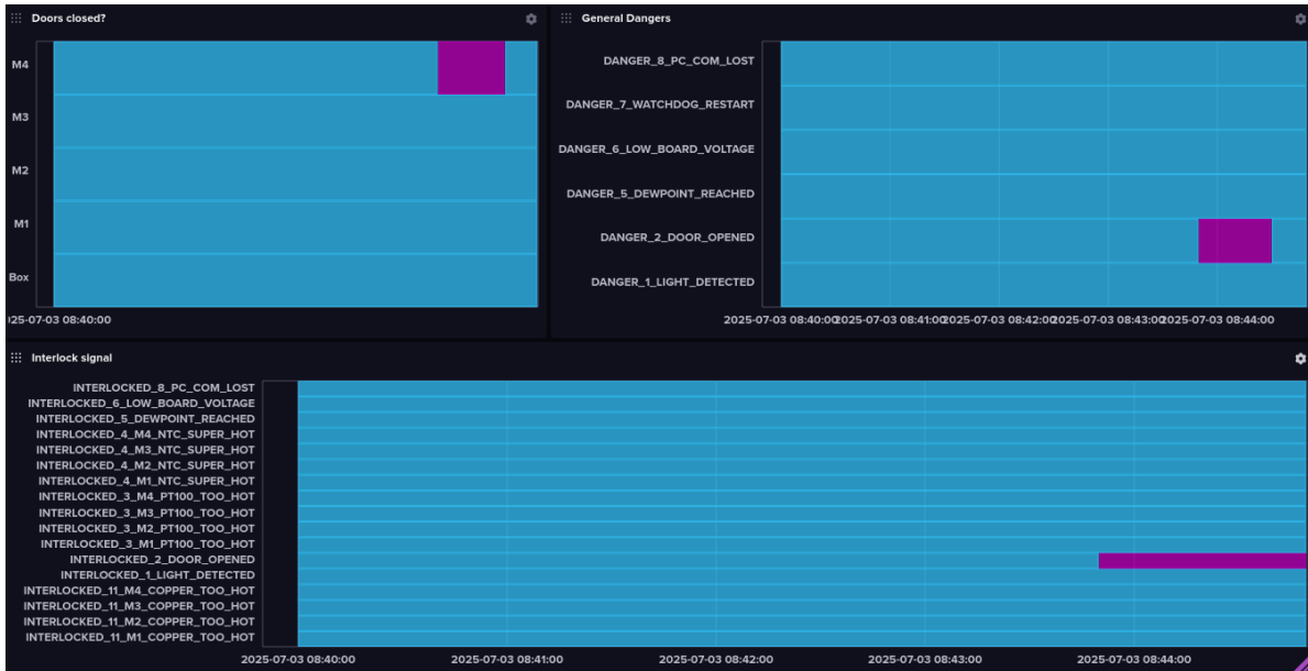
Figure 4.18: An interlock reaction to the opening of a door switch displayed in the influxdb to validate the interlock system.
