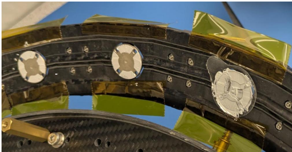
Figure 6.19: Front side of the Half-Ring with the Base Blocks covered with thermal paste with and without the thermal paste cover foil removed.
