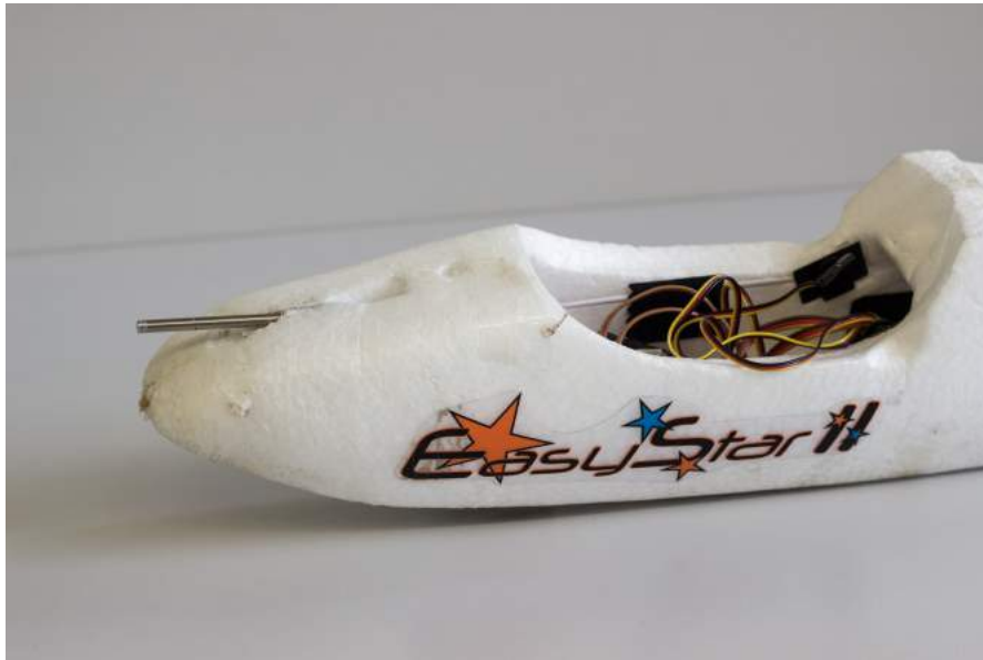
Figure 5.10: Pitot tube fixed on the nose of the drone.
