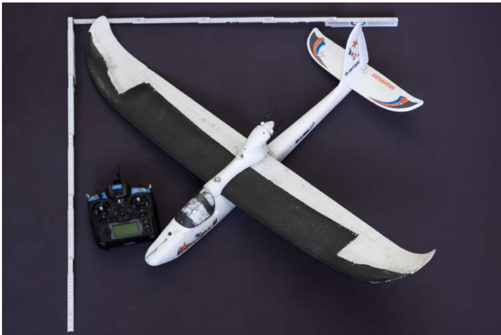
Figure 5.11: Complete Wind Drone.
