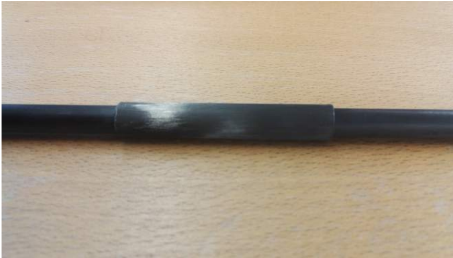
Figure 5.3: Two nested carbon tubes.
