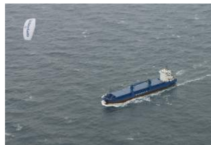
Figure 2.6: SkySails towing kite system in operation [17].
