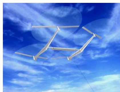
Figure 2.8: Flying Electric Generator (FEG) from Sky WindPower [22].
