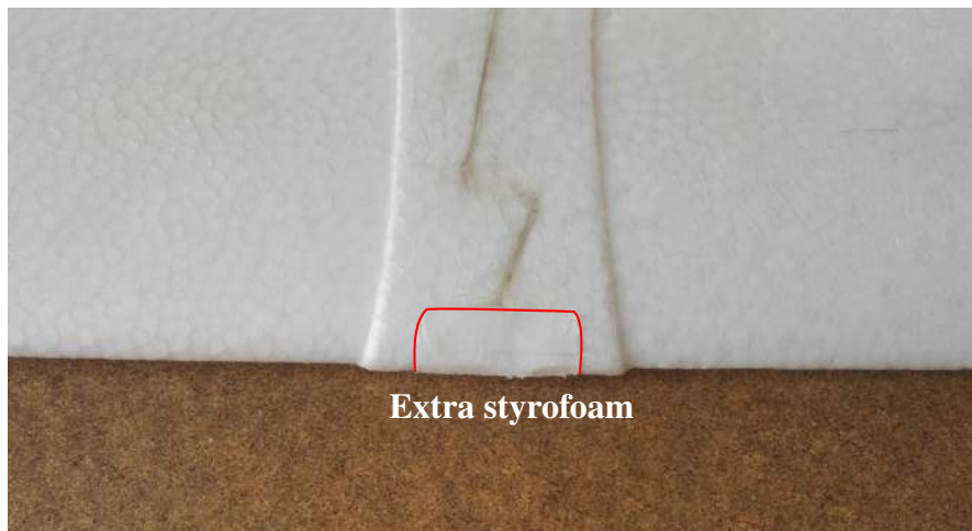
Figure 5.4: Glued wing parts with extra styrofoam in the recess.
