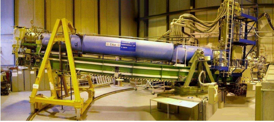
Figure 2.8: Photo showing the CAST experimental area, taken from [6]. The (shielded) x-ray detectors are mounted at the ends of the magnet.
