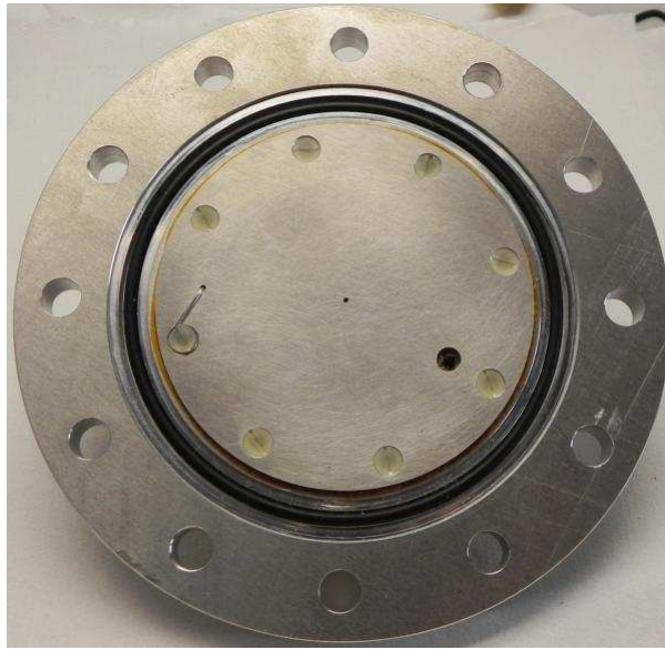
Figure 5.3: Picture of the top part of the detector as seen from inside. Cathode plate with x-ray window in its middle can be seen as well as the high voltage connection for the cathode (top left) and the gas outlet (down right).
