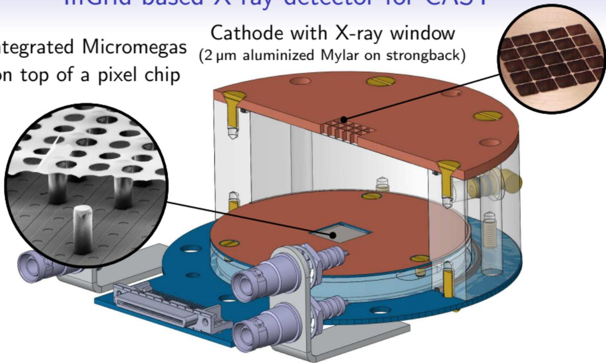
Drift volume flushed with  $\text{Ar}/i\text{C}_4\text{H}_{10}$  97.7/2.3
