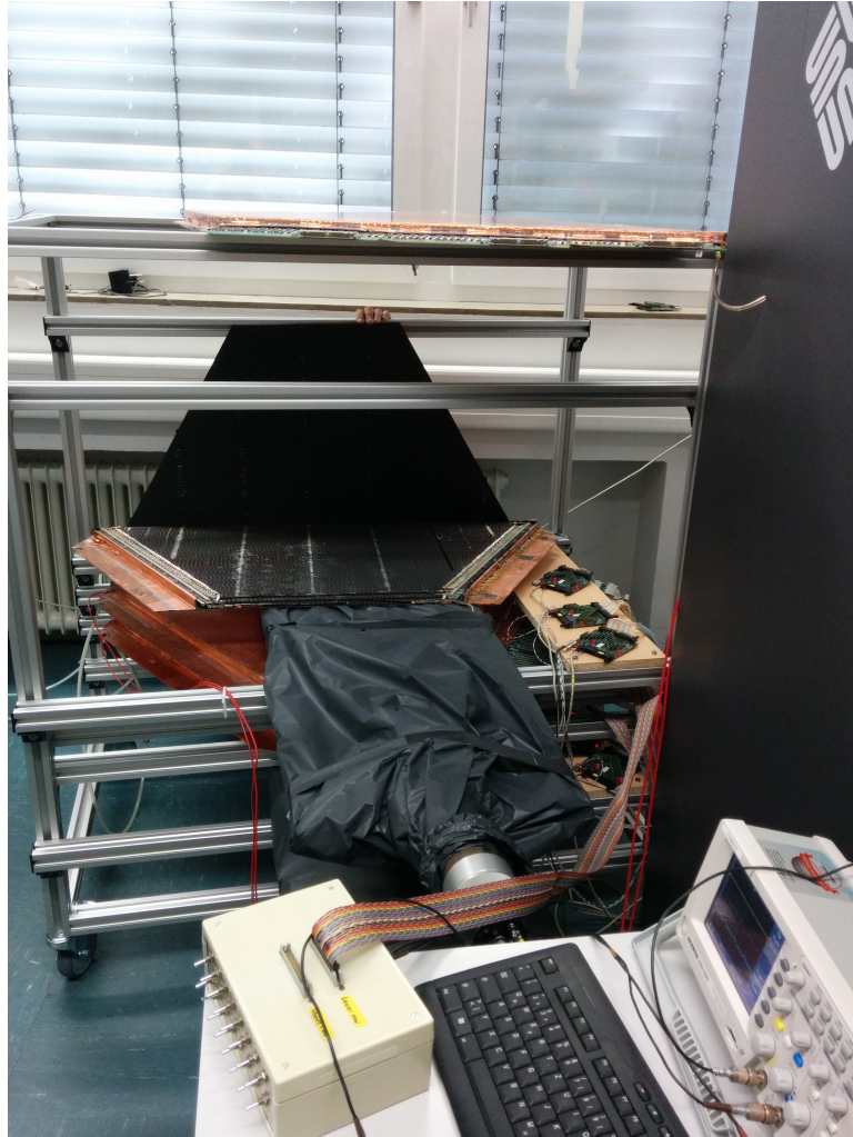
Figure 5.1: Test pulse setup used for testing hardware of the experiment. The ribbon cable from FE boards is connected to the switch box. From the switch box the signal is displayed on the oscilloscope.
