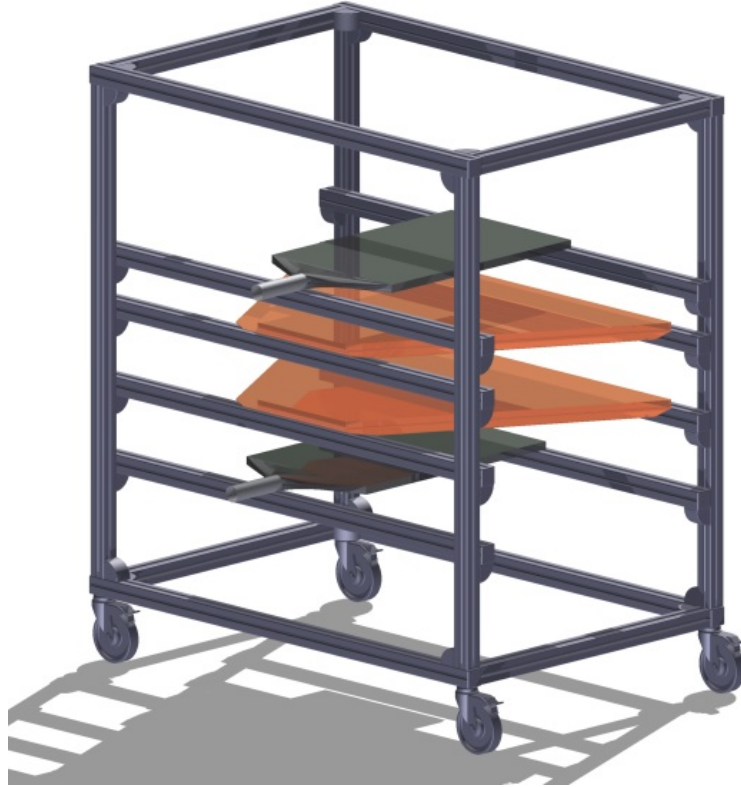
Figure 4.17: Schematic setup of the experiment with two modules (copper colored triangles) and two scintillators (black rectangle) with attached PMT (metallic tubes) as the trigger system.
