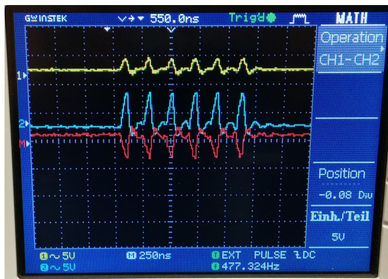
Figure 5.3: Test pulses in a problematic channel at STYX in Bonn. Blue and yellow lines are the signal from the ribbon cable, red line is the addition of both, blue and yellow, lines. The signal from one of two channels (yellow line) is deranged and the blue line shows extra peaks.
